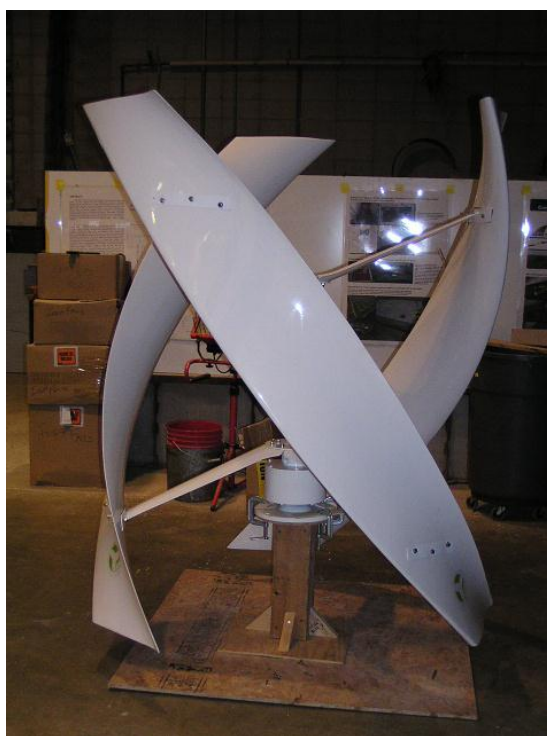
Figure 37: Full Assembly of 600 watt VAWT
